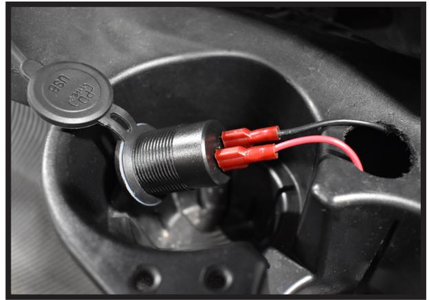
Insert USB into mounting hole and secure with the ring nut.
